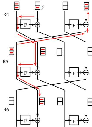
**Fig. 6.**  $\nabla_j$  difference injection in Round 4 and its propagation.
