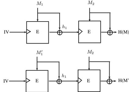
**Fig. 9.** Collision Attack.
