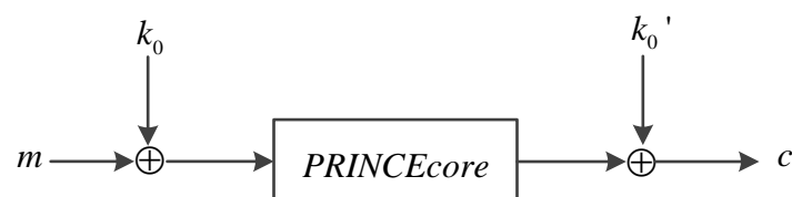
Fig1. The construction of PRINCE
