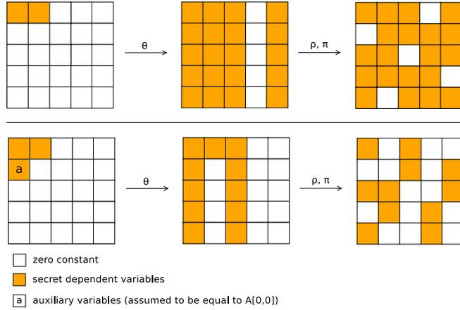
**Fig. 3.** Impact of auxiliary variables on diffusion of the secret key variables. When using auxiliary variables,  $A[0, 0]$  (secret variables) and  $A[0, 1]$  (auxiliary variables) are diffused to  $A[0, 0]$  and  $A[1, 3]$ , without affecting many lanes of the state.
