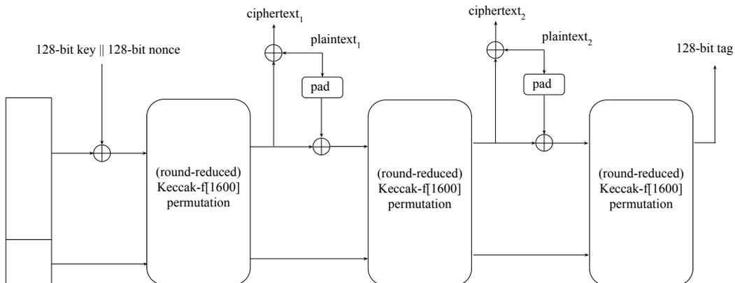
**Fig. 2.** Lake Keyak processing two plaintext blocks.
