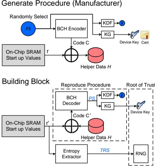
**Figure 4: The Generate Procedure and Building Block**
