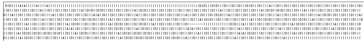
Fig. 3: FLUSH+RELOAD spy output. Vertical bars indicate time-slot boundaries; ‘A’ and ‘D’ are probes for OpenSSL access to add and double; dashes indicate missed time-slots.
