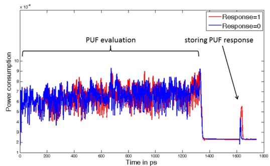
Fig. 3. Two power traces of an 128-bit Arbiter PUF for two different challenges, one challenge with a response of 1 and one with a response of 0.
