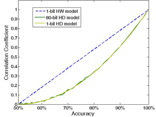
Fig. 8. Relation between the correlation coefficient and the prediction accuracy for the Hamming weight power model as well as the Hamming distance power model. For this simulation 1 million random response bits were used and no noise was added.
