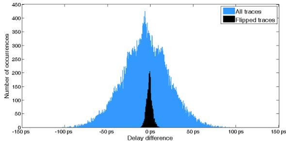
Fig. 11. The delay difference in pico seconds between the top and bottom signal after the last stage for 49k traces. Colored in blue are the delay differences of all traces and in black are the delay differences for the traces whose output flipped when the supply voltage was changed from 1.1V to 1V and 1.2V.
