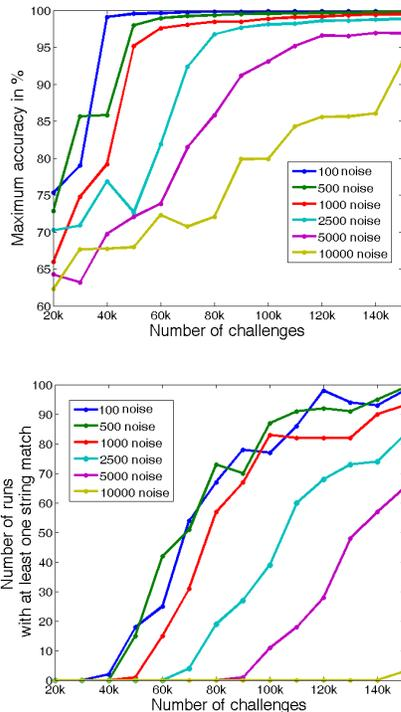
Fig. 9. Result of 100 runs of an 80-bit CCMA-ES attack with different levels of noise. The noise level is expressed by the number of randomly switching registers that would generate the same amount of noise. On the left the maximum achieved accuracy with 100 runs is shown while on the right the number of runs that achieved an accuracy high enough to find at least one string match is shown.
