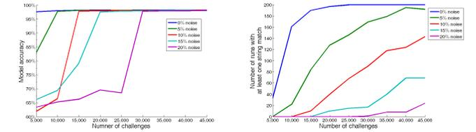
Fig. 14. Result of a Fault CMA-ES attack with 200 independent runs for different levels of overall-noise and for different numbers of challenges. On the left the highest achieved model accuracy is shown while the right figure shows the number of runs that had at least one string match.
