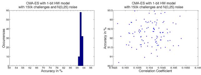
Fig. 5. Result of a CMA-ES with a 1-bit HW power model, 150k challenges and a noise of  $\mathcal{N}(0, 25)$  which is equivalent to 100 switching registers.
