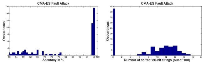
Fig. 12. The result of 100 runs of the CMA-ES Fault attack with 8k traces and  $\pm 0.1V$  supply voltage variation without additional noise. On the left the accuracy of the resulting PUF models are shown. On the right side the number of 80-bit strings that were correctly predicted by the PUF models are shown.
