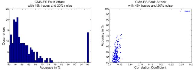
Fig. 13. The result of 100 runs of the CMA-ES Fault attack with 45k traces and  $\pm 0.1V$  supply voltage variation with 20% faulty responses.
