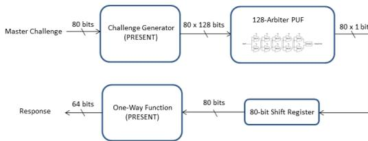
Fig. 2. The controlled PUF design. An 80-bit master challenge is applied to the controlled PUF from which 80 individual sub-challenges are derived using the challenge generator. These 80 sub-challenges are applied to the 128-bit Arbiter PUF and the 80 PUF responses are stored in a shift register. This 80-bit string is hashed using a cryptographically secure one-way function and the resulting 64-bit hash value is provided as the final response of the controlled PUF.
