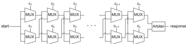
Fig. 1. Schematic of an n-bit Arbiter PUF.
