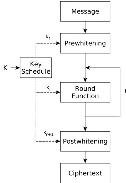
Figure 1: General Structure of An Iterative Block Cipher
