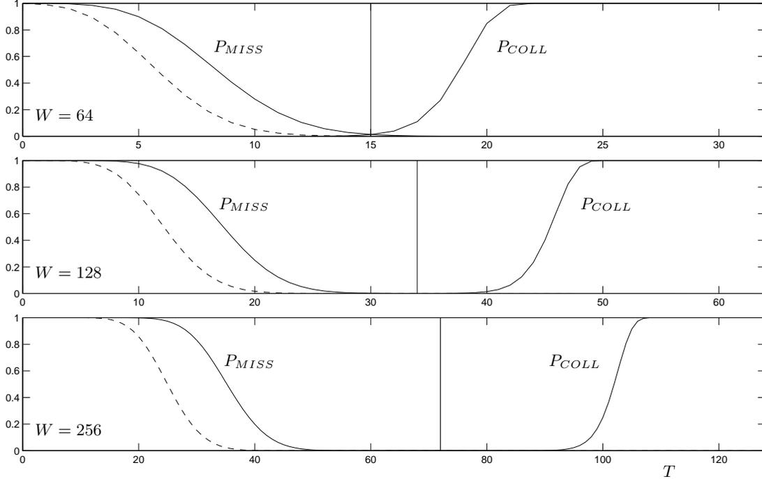
**Fig. 5.** Failure probabilities, incorporating our PUF statistics  $\overline{P_{MISS\_BIT}} = 0.14$  and  $\overline{P_{COLL\_BIT}} = 0.50$ , using  $L = 1024$  and  $W \in \{64, 128, 256\}$ . Functions are of discrete nature, although drawn continuously. The optimal thresholds are  $T = 15$ ,  $T = 34$  and  $T = 72$ . Dashed curves represent the pattern miss probability in case of a perfect majority vote:  $\overline{P_{MISS\_BIT\_IDEAL}} = 0.10$ .
