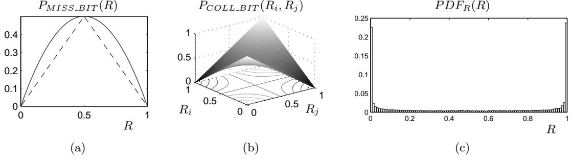
**Fig. 4.** (a) Probability of a response bit mismatch. The dashed curve corresponds with a majority vote during enrollment, in the ideal case. (b) Probability of a response bit collision. (c) Probability density function of  $R$  for our 65nm PUF.
