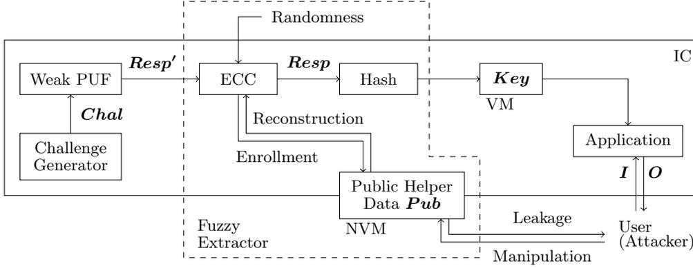
**Fig. 2.** Key generation via a typical fuzzy extractor
