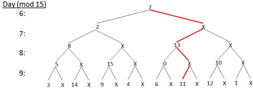
Figure 2: The routing tree of 7 from day  $d = 6 \pmod{15}$  according to the GLS in Figure 1. The X symbol signifies holding of the message. The bold lines are example to the routing procedure if 7 wants to send a message to 11: 7 holds the message one day and then forwards it to 13. 13 holds the message one more day, and forwards the message to 11 on day  $d + 3$ .
