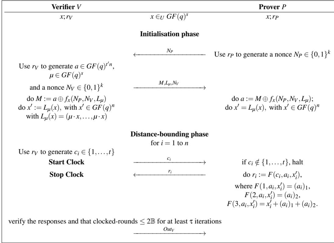
**Fig. 3.** The **SKI<sub>pro</sub>** Distance-Bounding Protocol ( $q = 2, t = 3, t' = 2$ )
