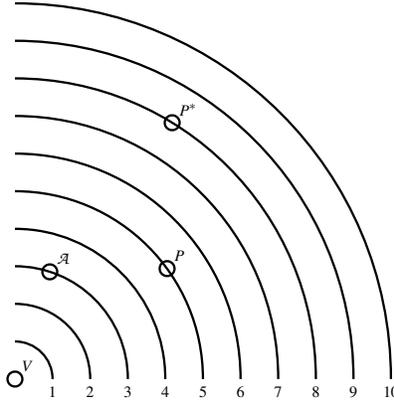
**Fig. 4.** Sketch of Message-Transmitting Model: A message send by  $V$  is broadcast and travels at one unit of distance per clock cycle. Assume  $P$  is the purported recipient. However,  $A$  can read the message two clock cycles before  $P$ , whereas  $P^*$  must wait three clock cycles more than  $P$  before the message reaches him.
