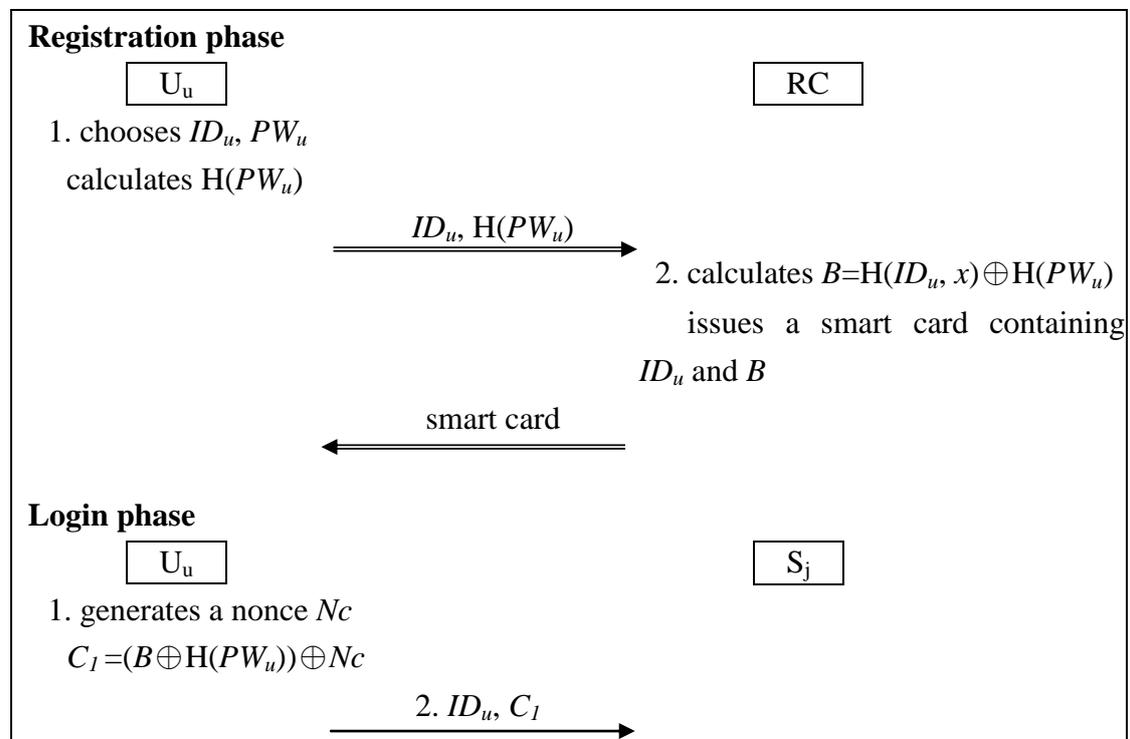
**Fig. 1. Registration phase and login phase of Tsai's protocol**
