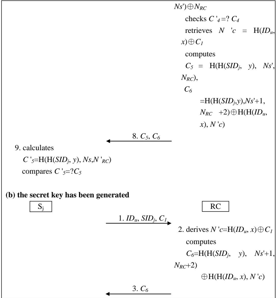
**Fig. 2. Authentication of server and RC phase of Tsai's protocol**
