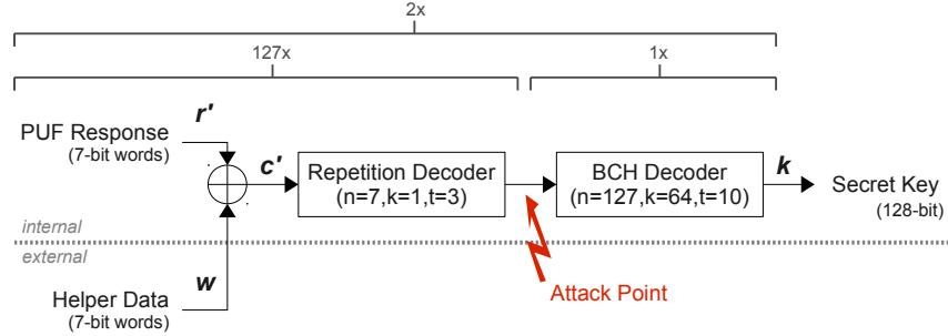
**Fig. 2.** Secure sketch implementation under test
