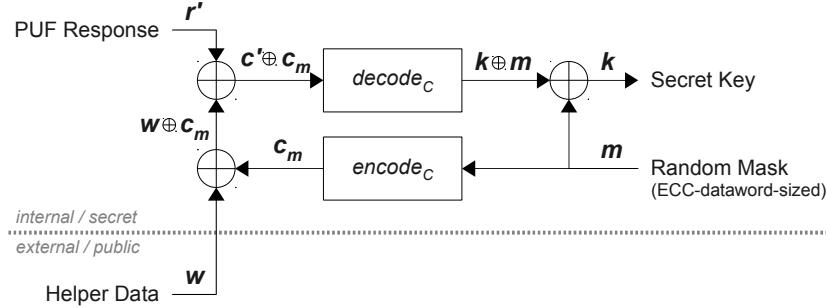
**Fig. 4.** Masked secure sketch (*Rec*)
