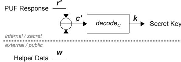
**Fig. 1.** Reconstruction module of a code-offset secure sketch
