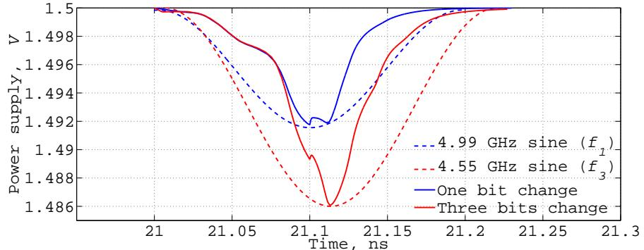
(c) Power consumption and sines with the frequency of the maximum spectral amplitude
