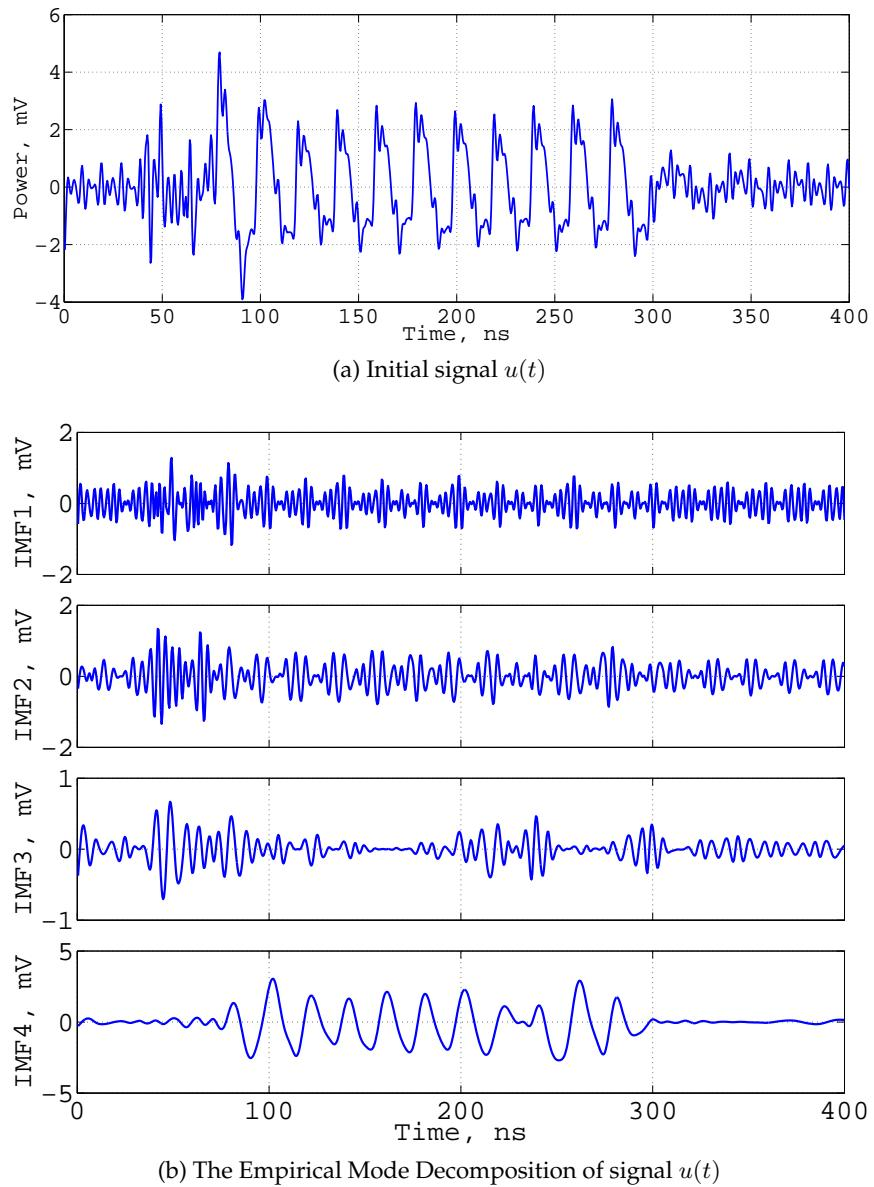
**Fig. 7.** Power consumption of our experimental AES-128 implementation.
