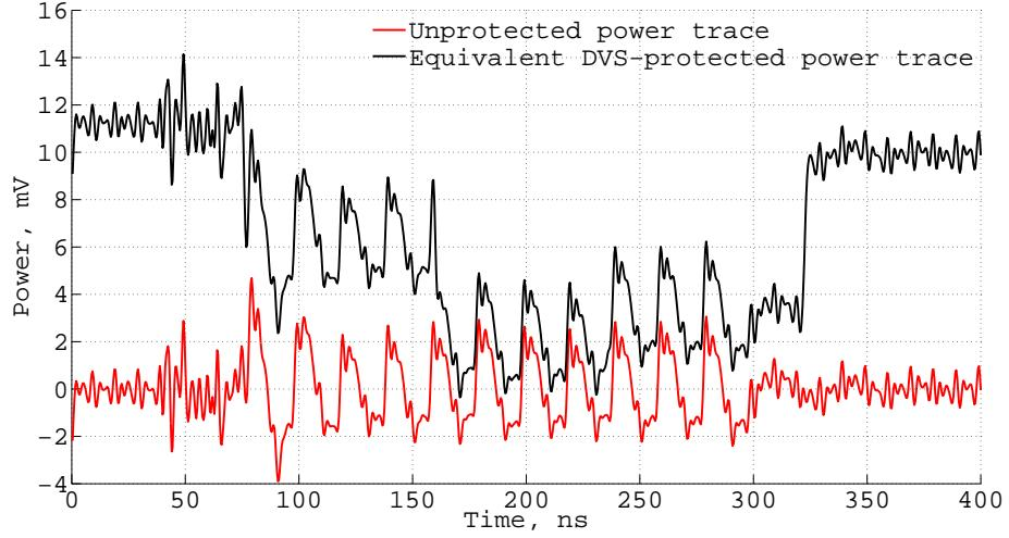
**Fig. 12.** Power traces of the FPGA AES implementation. The unprotected signal is shown in red. The DVS-protected signal is shown in black.
