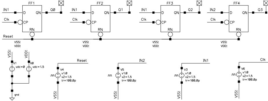
**Fig. 5.** Netlist of a 4-bit register.
