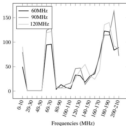
**Fig. 4.** Evolutions of the Mean Guessing Entropy on the frequency range:  $[0; 210MHz]$  after the processing of 60000 traces. The target design has been successively clocked at 60 MHz, 90 MHz and 120 MHz.
