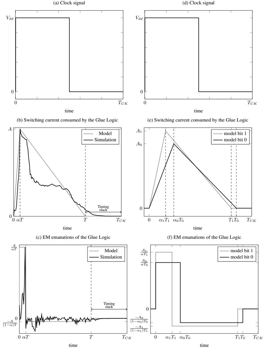
**Fig. 2.** Models of the switching current consumed (b) by the Glue Logic and of its EM emanations (c); Models of the current and EM leakages (e and f respectively)
