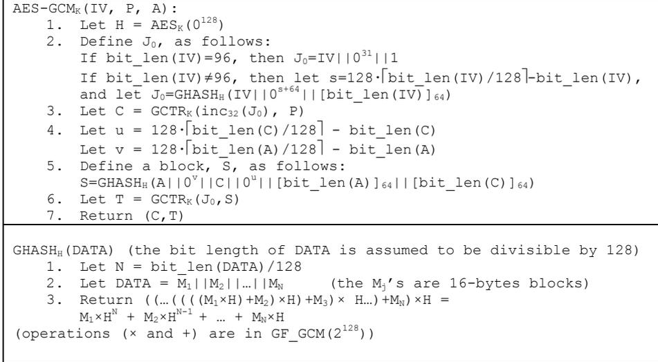
**Fig. 1.** Top panel: AES-GCM flow. Bottom panel: GHASH calculation (for a buffer whose byte length is divisible by 16).
