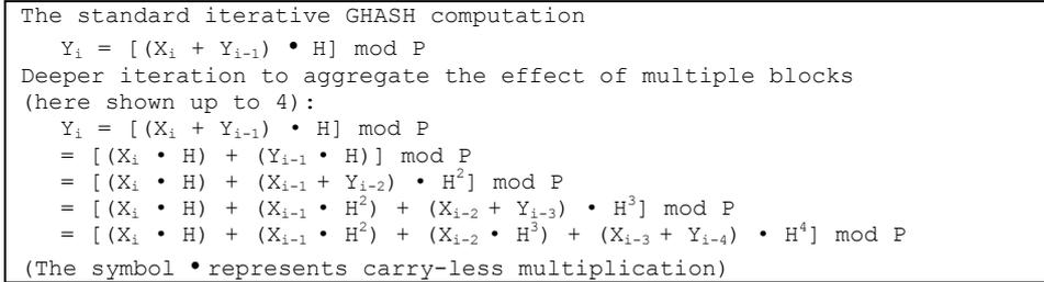
**Fig. 2.** GHASH optimization: deferring the reduction modulo  $P$  step, by aggregating (via carry-less multiplications) the cumulative contribution of several data blocks.
