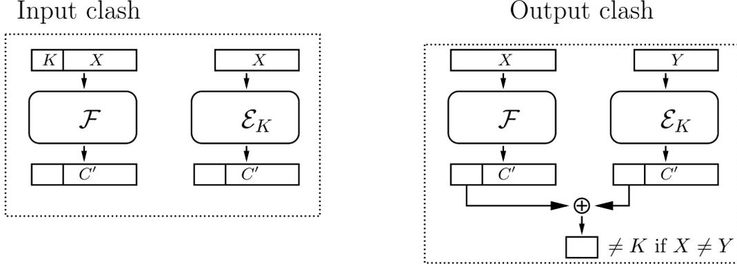
Figure 4: Detection and exploit of the clashes. In case of input clash we encrypt  $(n - k)$ -bit suffix  $X$  of the permutation query  $K||X$  and detect suffix collision in outputs. In case of output clash some ciphertext prefixes are forbidden, which allow to distinguish the encryption from the ideal cipher.
