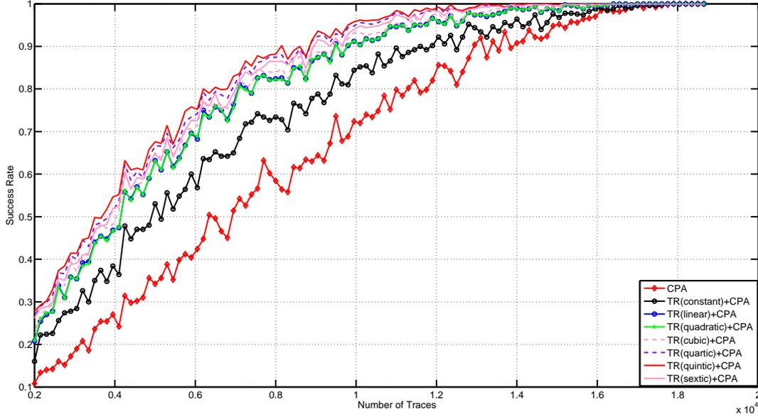
**Fig. 4.** CPA Attacks on Original Traces and on the Same Traces after Trend Removal with Different Polynomial Degrees
