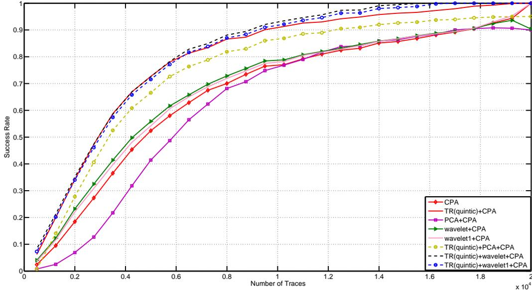
**Fig. 6.** CPA Attacks on Real Power Traces with Different De-noising Methods
