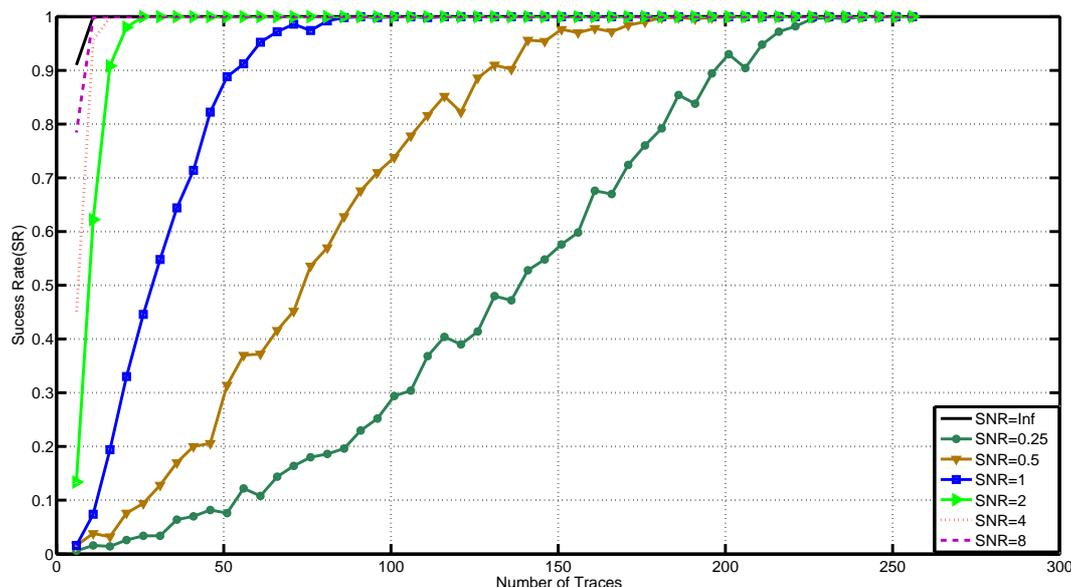
Fig. 5. CPA Attacks on Simulated Traces with Different Levels of Trend Noise
