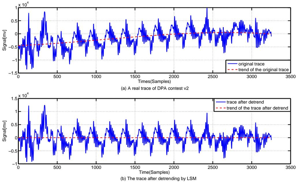
**Fig. 2.** One Real Trace in DPA Contest v2 and Its Corresponding De-trended Trace by LSM
