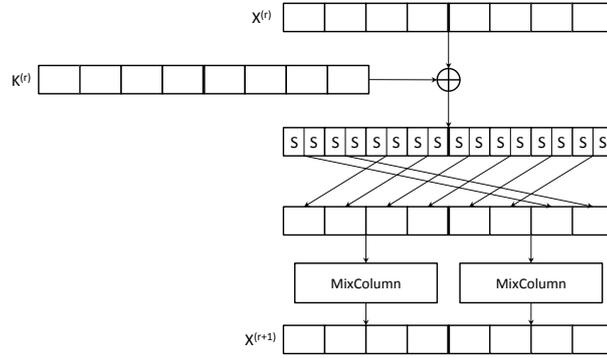
**Fig. 1.** One round of KLEIN block cipher
