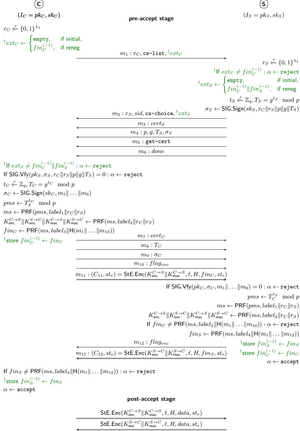
Figure 4: TLS handshake for TLS\_DHE\_DSS\_WITH\_3DES\_EDE\_CBC\_SHA ciphersuite with client authentication  $\dagger$  and SCSV / RIE renegotiation countermeasures
