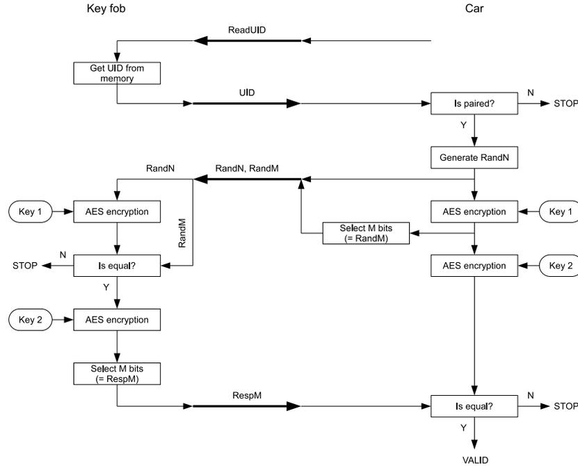
**Fig. 1.** “Bilateral authentication” between key fob and car.
