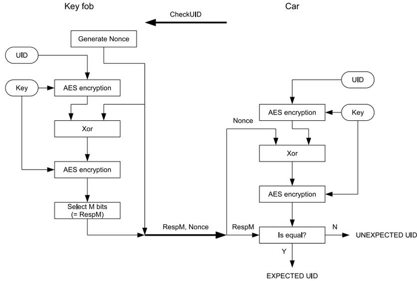
Fig. 3. Enhanced “CheckUID” command with resistance against tracking.
