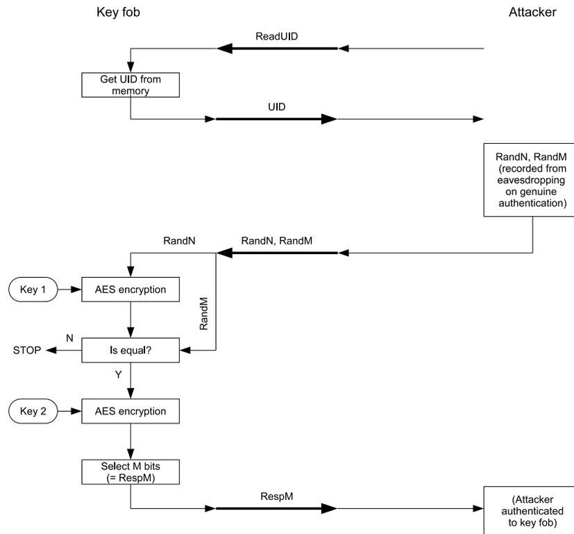
**Fig. 5.** Replay attack on the key fob.
