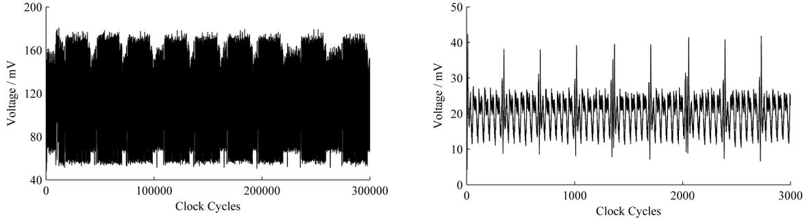
**Fig. 1.** Example power consumption trace showing the individual field multiplication operations in a group operation for the ARM7 (upper) and Virtex-II (lower) implementations.
