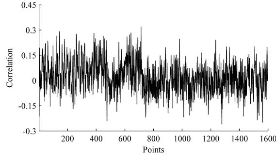
**Fig. 2.** An example correlation trace showing the correlation across one operation assuming that a collision occurs in every loop of the exponentiation. The example is generated from one power consumption trace taken while a Virtex-II FPGA was computing an exponentiation using Joye’s add-only exponentiation algorithm.
