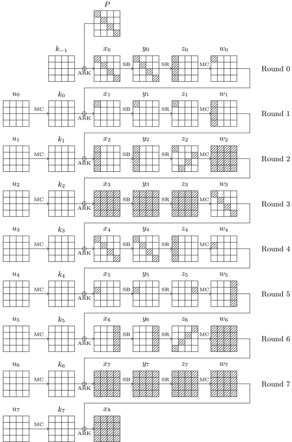
**Figure 8:** Complete 8-round truncated differential characteristic used in the attack of [Section 4.1](#).
