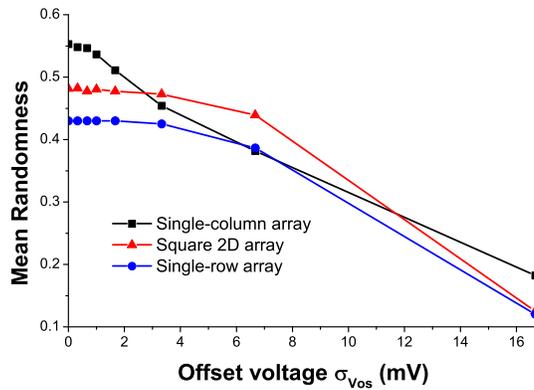
Figure 12: Dependence of randomness on offset voltage spread.
