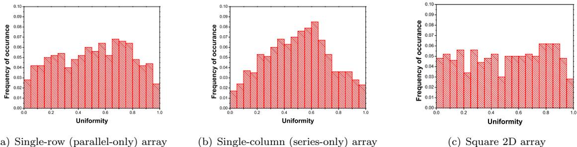
**Figure 7:** Distribution of the uniformity metric for three array topologies.
