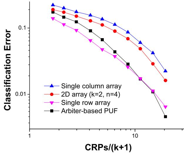
Figure 8: Classification error from modeling an 8-bit PUF via an SVM-based attack.
