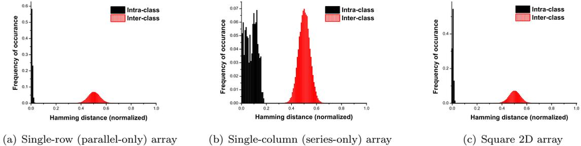
**Figure 6:** *Inter-class and intra-class HD for three array topologies.*
