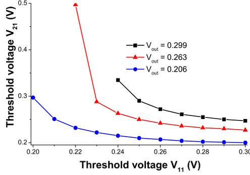
**Figure 5:** Response nonlinearity in the  $2 \times 2$  SCA.
