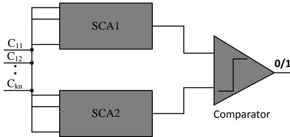
Figure 1: PUF architecture.
