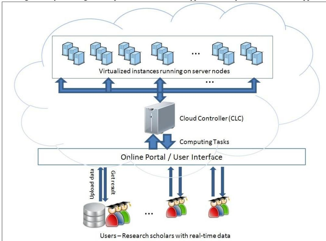
Figure 1. Basic Structure of A Typical Cloud Computing System for Scientific Applications
