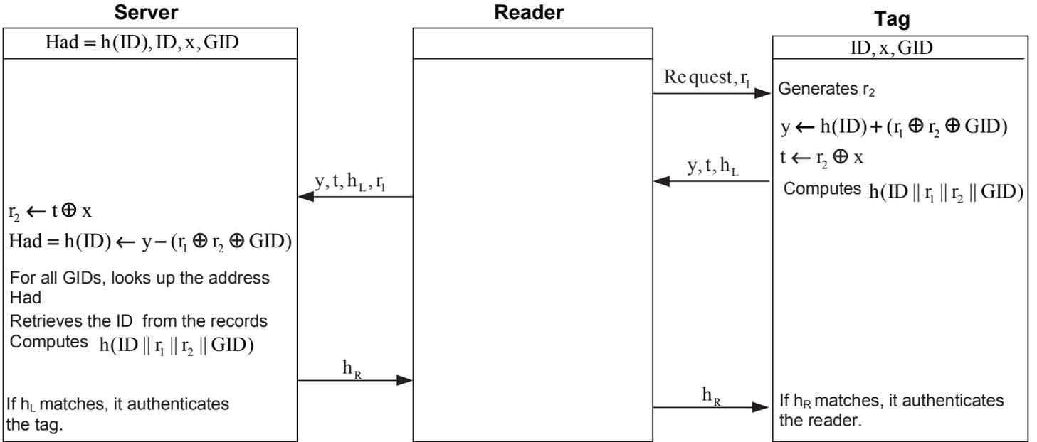
Fig. 2. SUAP2 authentication protocol proposed by Morshed *et al.* [8].
