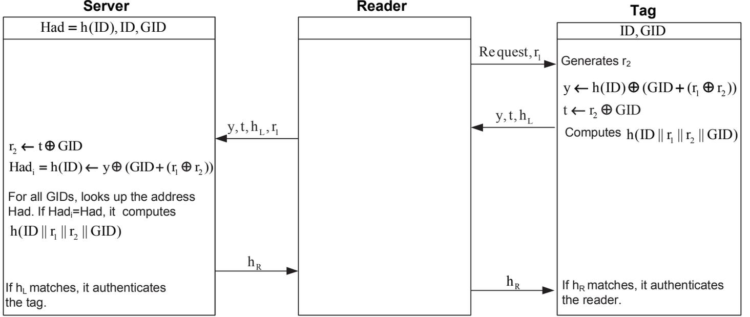
Fig. 3. SUAP3 authentication protocol proposed by Morshed *et al.* [8].
