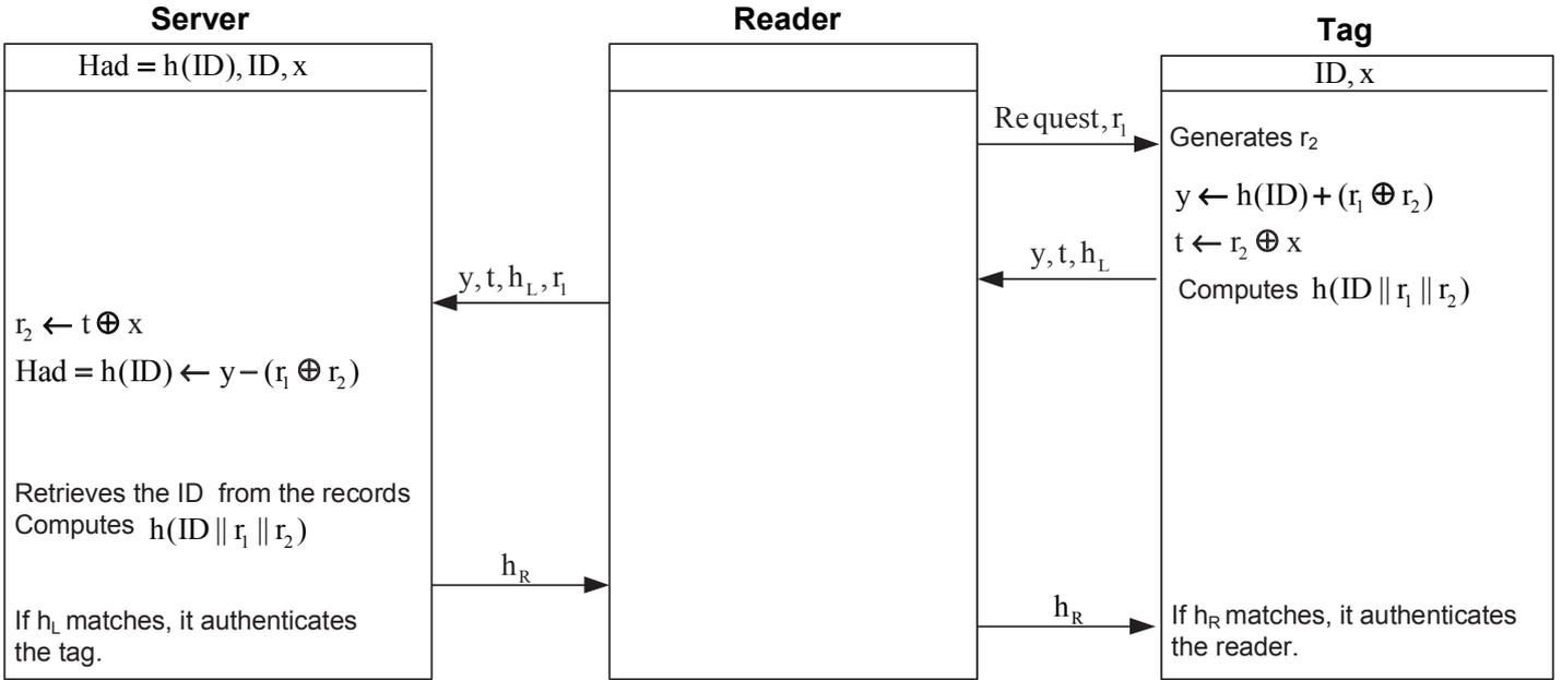
Fig. 1. SUAP1 authentication protocol proposed by Morshed *et al.* [8].
