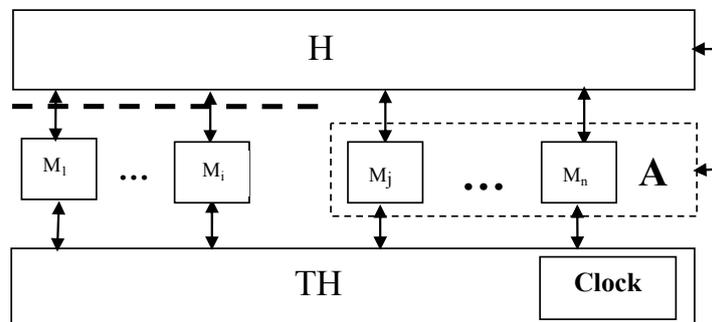
Fig.4. Clock is a part of the trusted host (ideal system)
