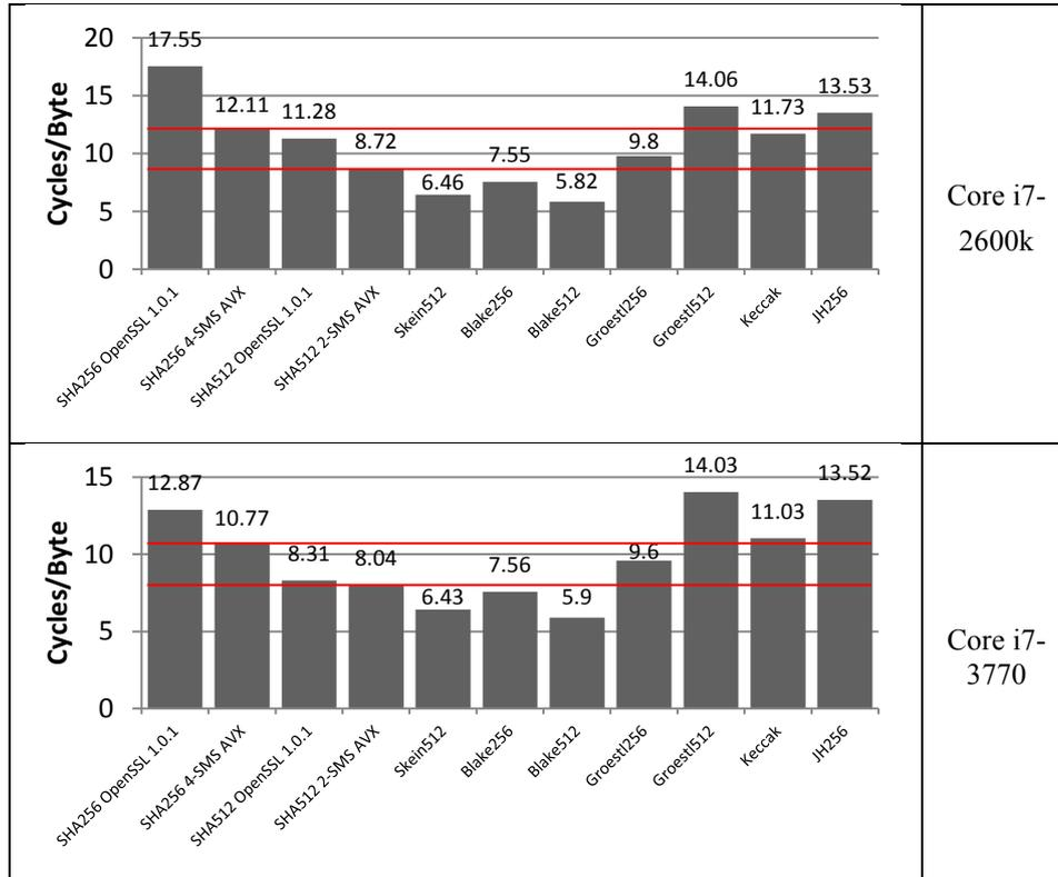
**Fig. 7.** Performance of SHA-256, SHA-512 and the five SHA3 finalists on the 2<sup>nd</sup> and the 3<sup>rd</sup> Generation Intel<sup>®</sup> Core<sup>™</sup> Processors. See details in the text. The horizontal lines show the new “performance bar” of SHA-256 and SHA-512 with the n-SMS method.
