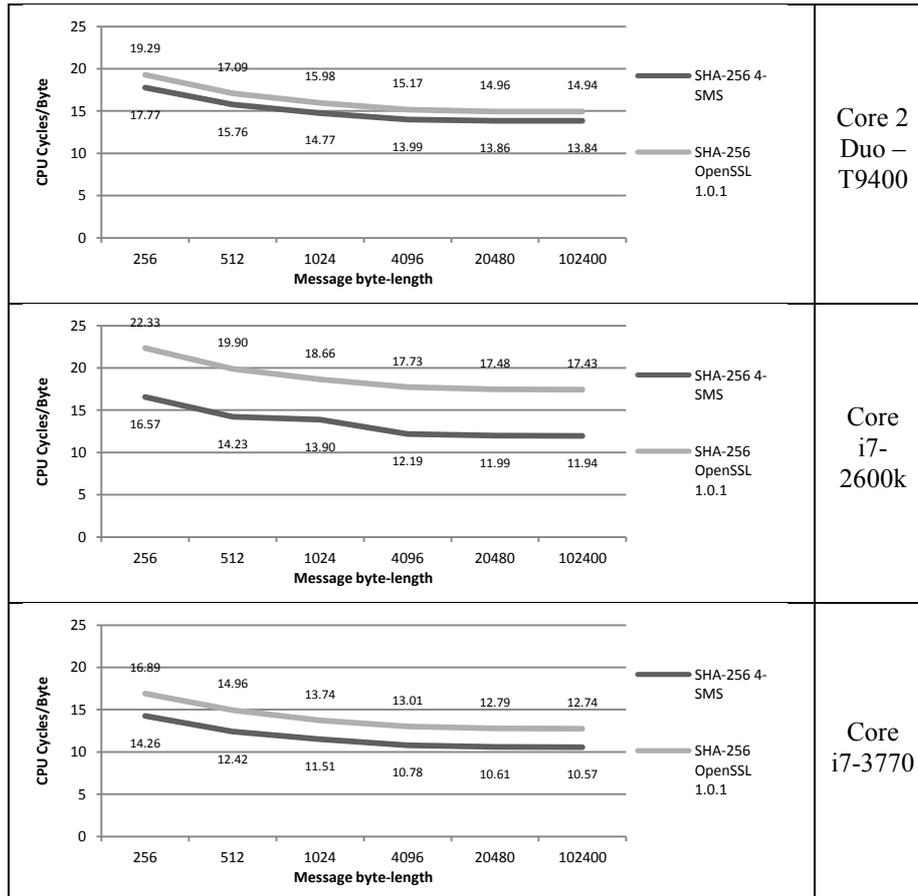
**Fig. 3.** Performance of SHA-256 on different processors and various message lengths.
