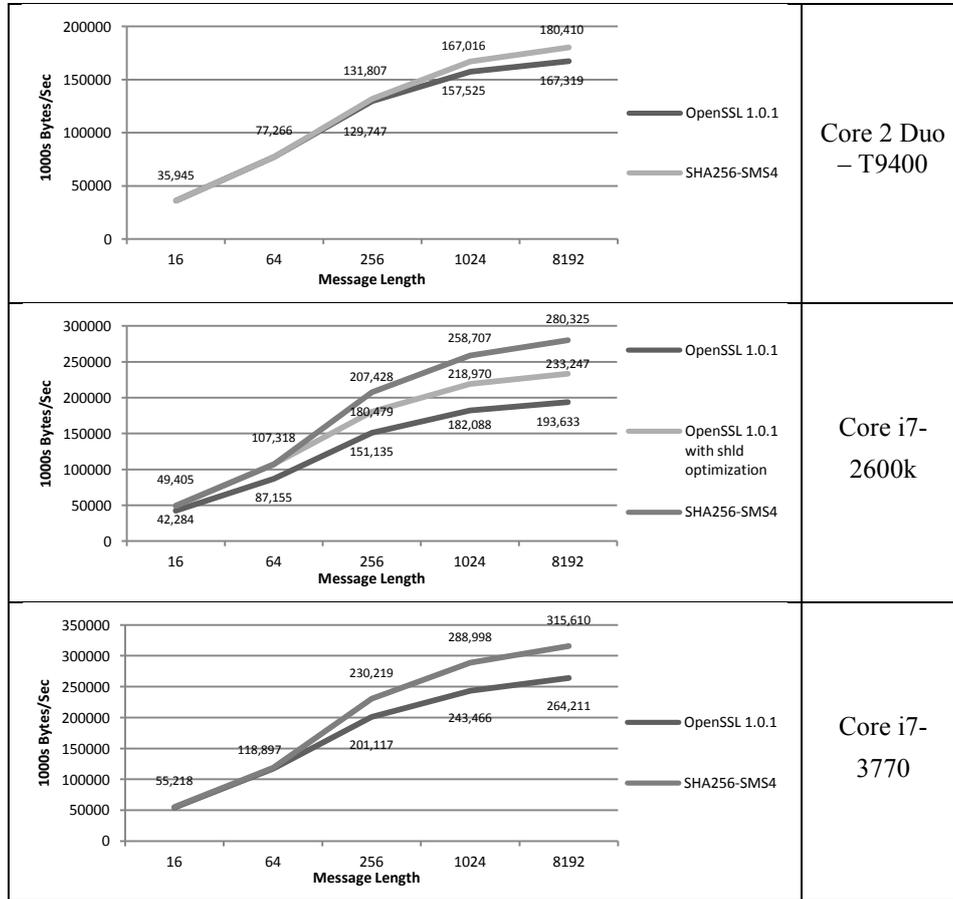
**Fig. 4.** Performance of SHA-256 as reported by the “openssl speed sha256” utility. Three variations were measured: 1) the original OpenSSL 1.0.1 implementation; 2) OpenSSL 1.0.1 with 4-SMS optimization [4]; 3) an optimized OpenSSL 1.0.1 implementation, obtained from using ‘shrd’ for rotation (instead of ‘ror’; see [2] for details)—relevant only for the 2<sup>nd</sup> Generation Core™. The performance is reported in 1000s bytes hashed per second (higher is better)
