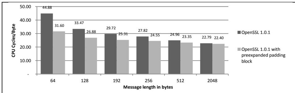
Fig. 6. Performance of OpenSSL 1.0.1 on a Core i7-3770 for short buffers, with and without the pre-expanded message schedule optimization, for the final block.
