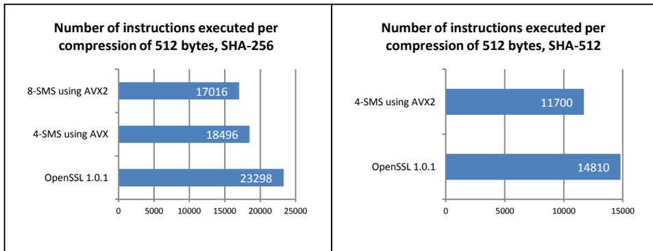
Fig. 5. Instruction count per compression of a 512 byte message block for different implementations
