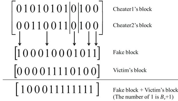
Figure 8: The process of this attack for the (2,3) better scheme.
