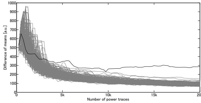
**Fig. 5.** The evolution of the lowest-mean test against the number of used traces.
