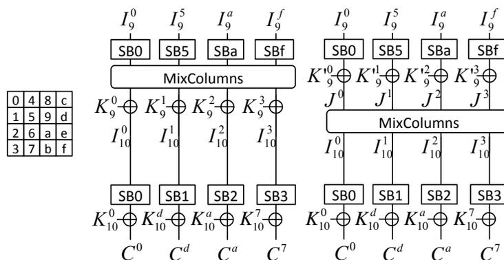
**Fig. 1.** Model of 4 bytes in the final 2 AES rounds.
