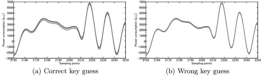
**Fig. 4.** Mean traces for 256 groups of power traces according to  $J^0 \oplus C^0$ .
