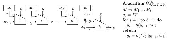
Figure 15: The CS (Chaining Shift) Construction
