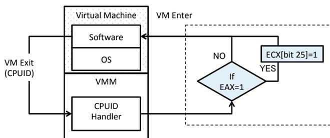
**Fig. 3.** How to fake CPUID
