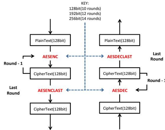
**Fig. 1.** AES-NI Encryption/Decryption Flow for AES-ECB mode
