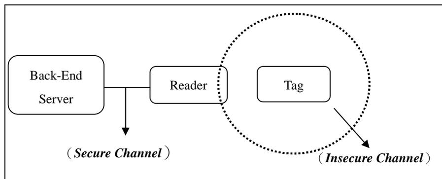
**Fig. 1. A typical RFID system**
