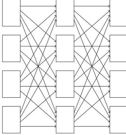
**Fig. 1.** A (4, 4, 4)-Clos network for implementing any permutation from  $S_{16}$
