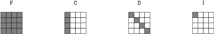
Fig. 3. Byte-wise truncated differential for an AES state. Each cell represents a byte and a gray cell stands for an active byte.
