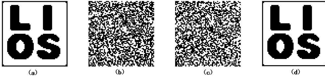
Figure 1: A 2 out of 2 VCS_{XOR} where (a) is the original image, (b) and (c) are the shares, (d) is the recovered image from (b) and (c).
