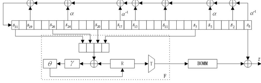
**Fig. 1.** The structure of Loiss
