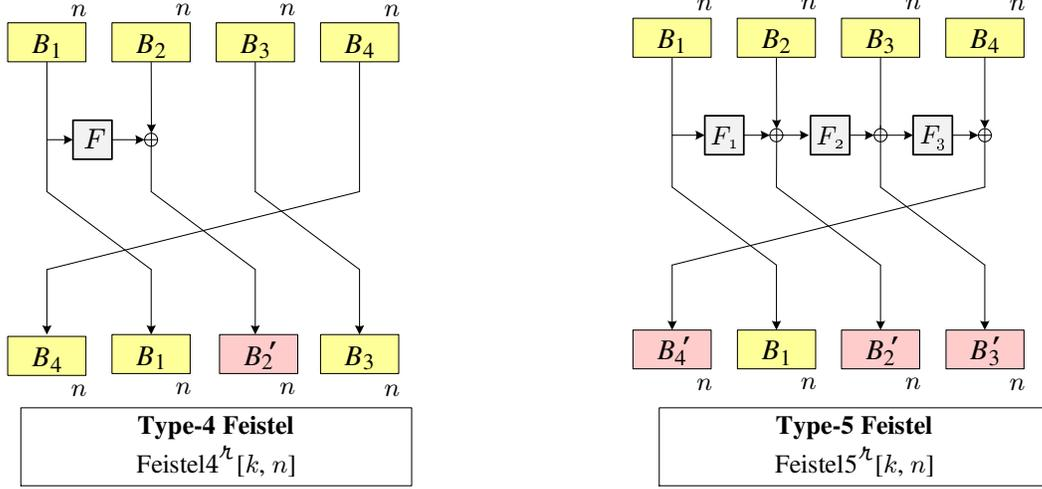
**Fig. 6. Type-4 and Type-5 Feistel networks.** The illustrations show a single round  $\mathcal{r} = 1$ , for  $k = 4$   $n$ -bit input blocks. Left is the Type-4 Feistel, and right is the Type-5 Feistel.
