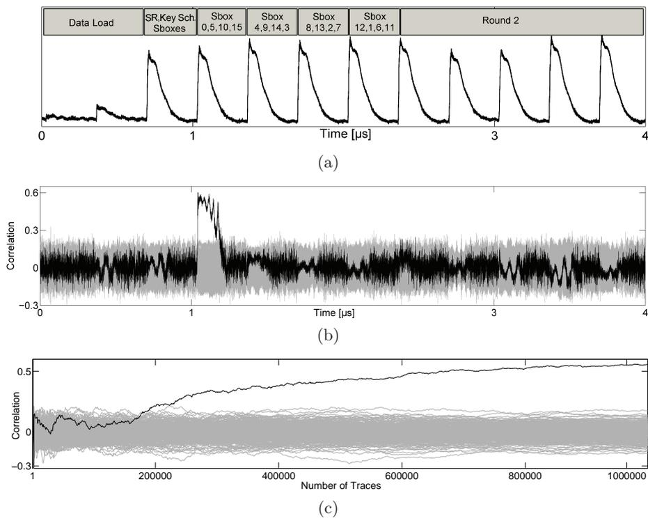
**Fig. 10.** (a) a power trace of the 32-bit architecture, (b) the result of collision attack using the mean traces of byte 0 and byte 4, and (c) the result of the attack over the number of used measurements
