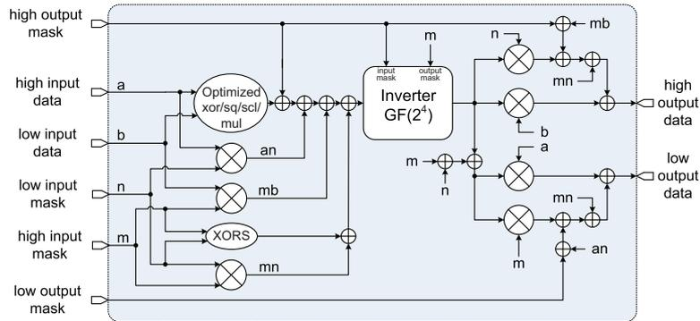
**Fig. 2.** Block diagram of the used masked  $GF(2^8)$  inverter
