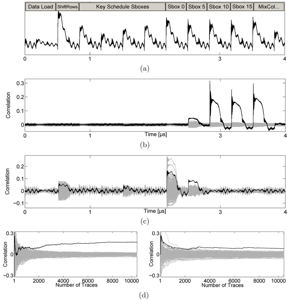
**Fig. 3.** (a) A measured power traces of an undefended implementation, (b) DPA attack result predicting toggles in the state register, (c) DPA attack using zero value model predicting the S-box input, and (d) the required number of traces in attacks using (left) HD model and (right) zero value model.
