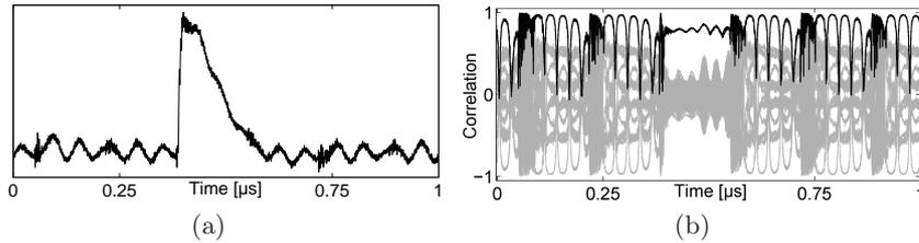
Fig. 9. (a) a power trace of the module under test, (b) the result of collision attack using the mean traces of the test module
