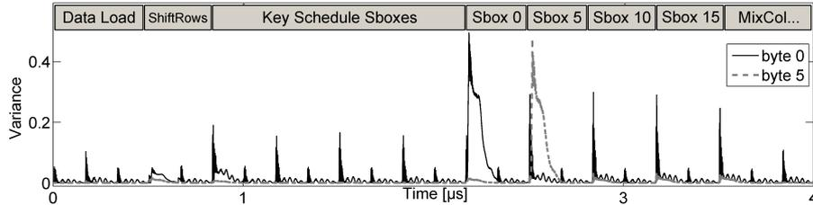
**Fig. 6.** Variance of mean traces for plaintext byte 0 and 5
