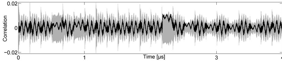
**Fig. 5.** Result of a zero value DPA attack on the masked implementation using 1 000 000 traces.
