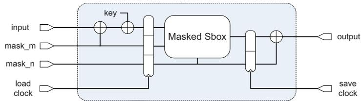
Fig. 8. Diagram of the test module
