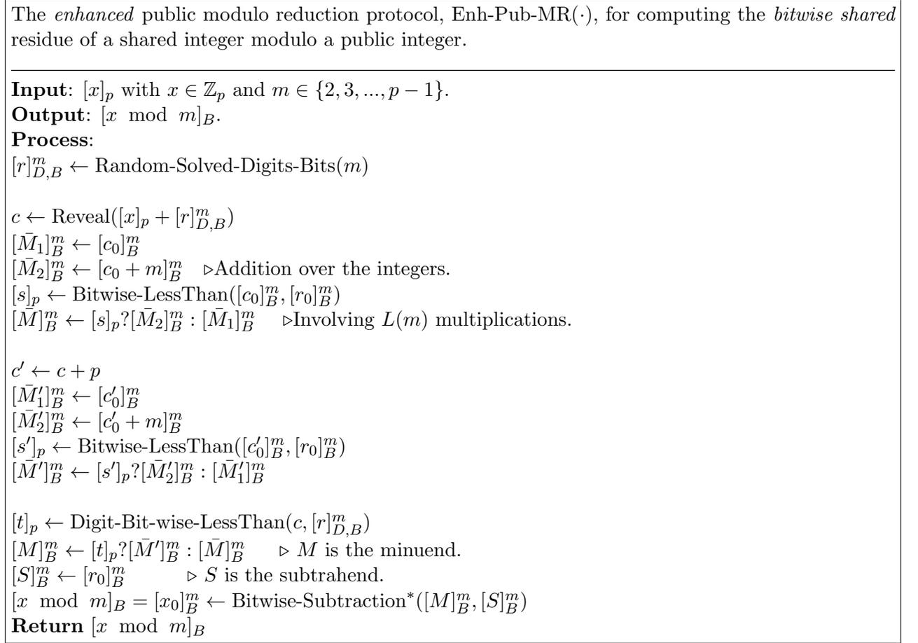
Figure 2: The *Enhanced* Modulo Reduction Protocol
