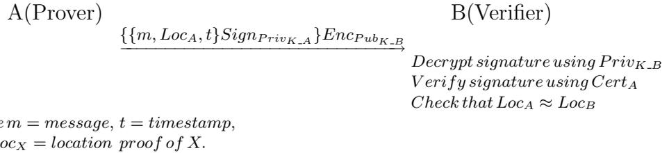
**Fig. 4.** An example of using location proof for preventing relay attacks in P2P NFC Transactions.
