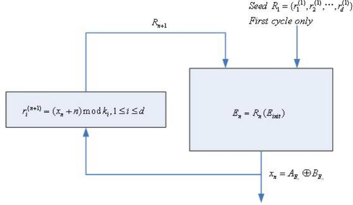
Figure 2: Block diagram of the proposed random number generator.
