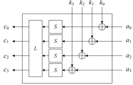
Fig. 2. The round function  $F$  of SMS4
