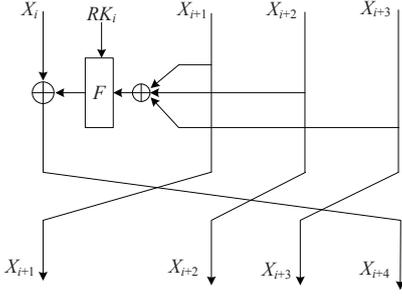
Fig. 1. The overall structure of SMS4
