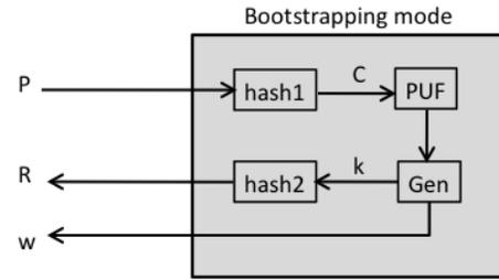
Figure 2: *Bootstrapping mode.* The control layer receives a pre-challenge  $P$ . The pre-challenge is hashed, yielding a challenge  $C$ , which is fed to the PUF. The PUF output is sent to the `Gen` function, which generates a secret key  $k$  and helper data  $w$ . The key  $k$  is hashed, yielding the response  $R$ . Finally, the control layer outputs the helper data  $w$  and the response  $R$ .
