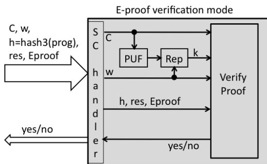
Figure 6: *E-proof verification mode*. The protocol is run through a SC. The CPUF recovers the secret key  $k$  from  $(C, w)$  by using the PUF and the Rep function. The VerifyProof module then verifies the consistency between Eproof, the key  $k$  and the data  $C, w, h, res$ .
