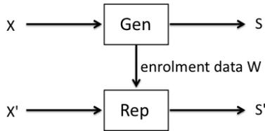
Figure 1: *Fuzzy Extractor*. The **Gen** function takes a measurement  $X$  as input, and generates helper data  $W$  and a near-uniform key  $S$ . The **Rep** function attempts to reproduce  $S$  from  $W$  and a noisy measurement  $X'$ . It succeeds ( $S' = S$ ) if the noise is sufficiently weak.
