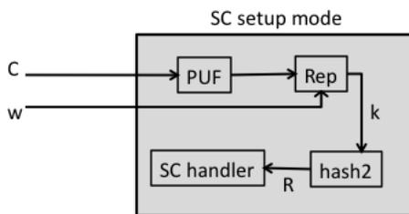
Figure 3: *Secure Channel setup mode.* The control layer receives  $C$  and  $w$ . It feeds  $C$  to the PUF. The PUF output and  $w$  are sent to the Rep function, which reproduces the key  $k$ . This gets hashed, yielding the shared secret  $R$ , which is then used by the ‘SC handler’ module to handle the secure communication channel with the user.
