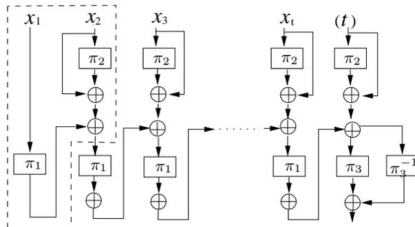
**Fig. 7.** The enhanced three-key enciphered CBC mode
