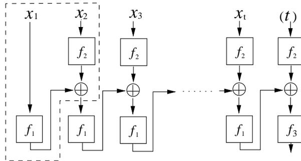
**Fig. 6.** The basic three-key enciphered CBC mode
