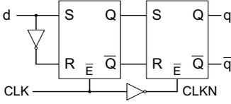
**Fig. 1.** Typical block diagram of an edge-sensitive flip-flop
