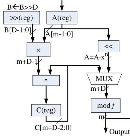
Fig. 1. Our Implementation of LSD-First Digit-Serial Multiplication Algorithm Over  $GF(2^m)$
