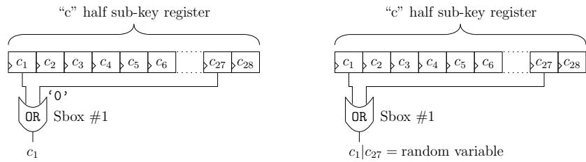
Figure 7: Consistent (left) and noisy (right) combinatorial logic driven by the “C” register.
