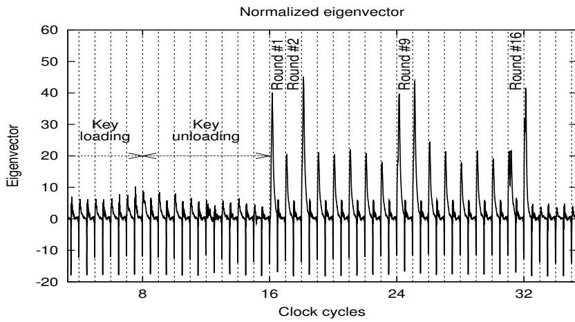
Figure 4: First eigenvector in campaign #1 with “identity”-based classification.
