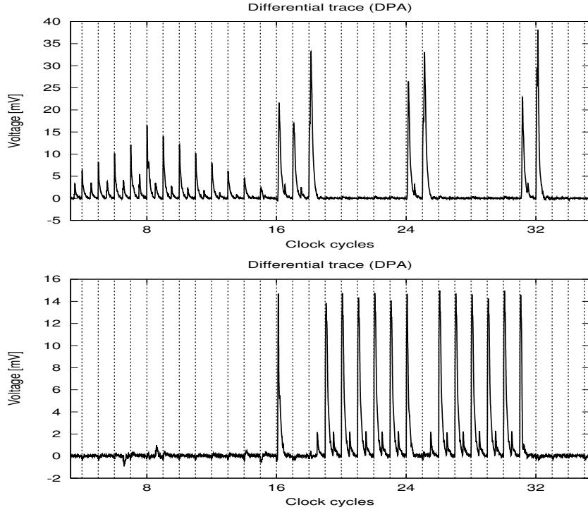
Figure 16: Differential traces obtained by traces weighting with  $\phi_1$  (upper) and  $\phi_2$  (lower).
