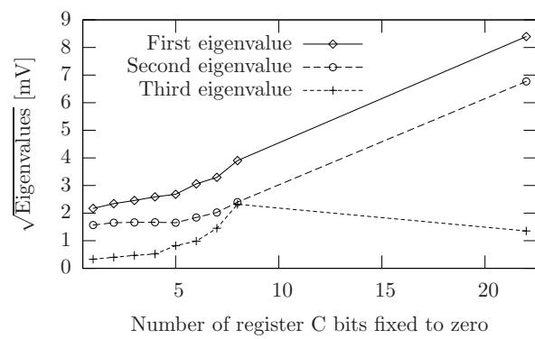
Figure 9: Three main eigenvalues when 1, 2, ..., 8 bits are forced to zero in the key.
