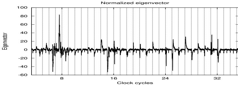
Figure 5: First eigenvector for the acquisition campaign #2 with “identity”-based classification.
