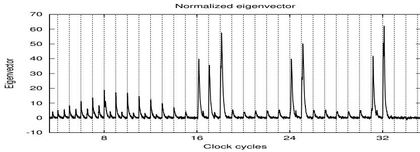
Figure 11: First eigenvector for the acquisition campaign #2 with  $\phi_1$ .
