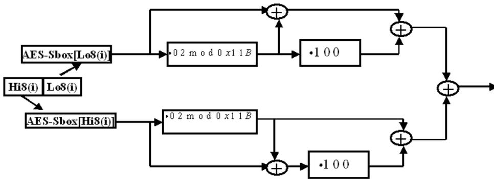
Figure 1. How to generate the S-box in TKIP
