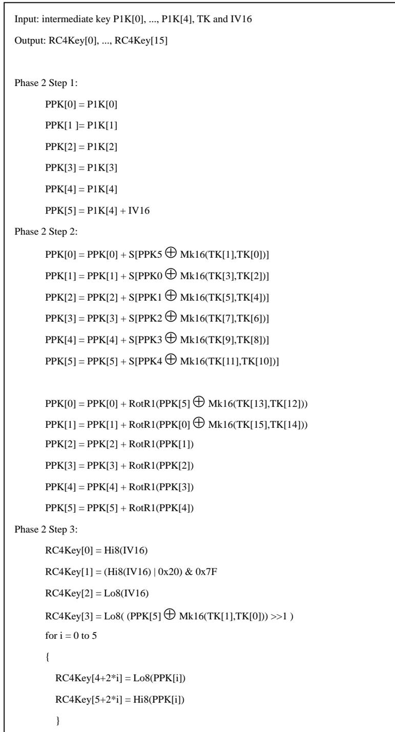
Figure.2 The Algorithm of Key Mixing Phase 2
