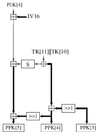
Figure 3. Part of Phase 2 needed to compute TK[10] and TK[11], cited from Refs.[14]
