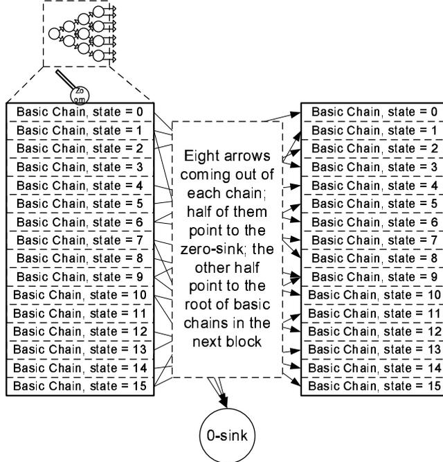
lead to the 0-sink, while the other half advance to appropriate states on the next block. Figure 4 illustrates the full structure of the OBDD representing the compressor.
