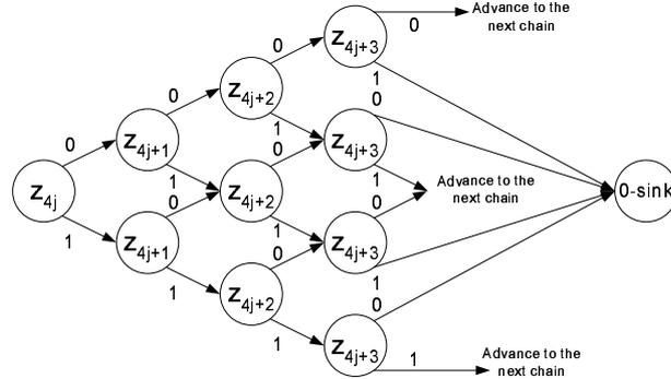
Fig. 4. Two consecutive blocks in an OBDD representing the compressor
