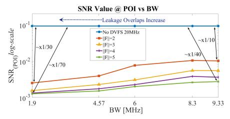
**Figure: 13.** SNR@POI values vs Bandwidth, a decrease by a factor of one to two magnitudes is achieved carefully selecting the BW to generate aliasing in the time-domain.
