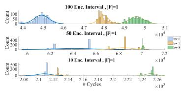
**Figure: 21.** Clock cycles measured over 100 encryptions, frequency changed with varying intervals. ||F|| = 1.
