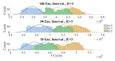
**Figure: 22.** Clock cycles measured over 100 encryptions, frequency changed with varying intervals. ||F|| = 3.
