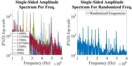
**Figure: 4.** FFT of different scenarios: (a) no randomization, single frequency  $f_n \in F'$ , ||F|| = 1 (b) Randomized scenario,  $f_n \in F$ , ||F|| = 7.
