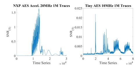
Figure: 10. SNR of the NXP AES accelerator to the left and the software Risc-V AES to the right under evaluation.
