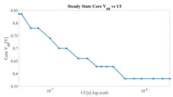
Figure: 5. Core voltage per 1/freq. available on our target device, PLS15
