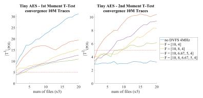
Figure: 16. Risc-V SW Tiny-AES: Maximum absolute values over time of a T-Test detection test based on TVLA methodology vs. the number of collected traces and for different ||F|| for a given BW(6MHz),  $V_{min} = 0.66[V]$ .
