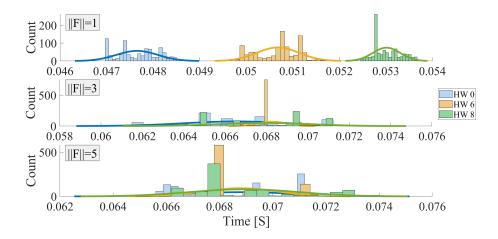
**Figure: 20.** Timing measured over 1K encryptions, performed with the same HW/freq./voltage. For a worst-case analysis, all plaintext bytes are the same for minimal noise. Measured with 10-100k traces per HW for increased ||F||.
