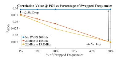
**Figure: 26.** Swapping from default 20MHz to a different core frequency for a percentage of the measured queries led to a reduction in the Corr POI value
