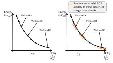
**Figure: 1.** DVFS conceptual implementation (a) insecure, single frequency per workload vs. (b) our proposed secure implementation, with multiple frequencies assigned per workload.
