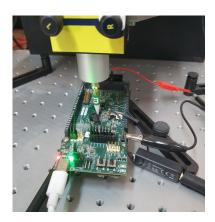
**Figure: 8.** Measurement setup with the PLS15 evaluation-board, the CT-1 current probe connected to a power jumper and the 0.1 mm Riscure's EM coil probe on top (tests were also performed with Langer's probes set).
