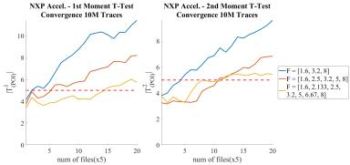
Figure: 17. NXP AES ACCEL.: Maximum absolute values over time of a T-Test detection test based on TVLA methodology vs. the number of collected traces and for different ||F|| for a given BW (5.4MHz),  $V_{min} = 0.58[V]$ .
