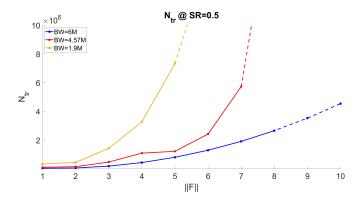
Figure: 19. Risc-V SW Tiny-AES: Number of traces required to achieve SR = 0.5 vs ||F|| across different BW, dashed line denotes curve extrapolation
