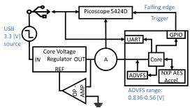
**Figure: 6.** Connection scheme of the core power supply and voltage regulation for the PLS15, with our current probe location.
