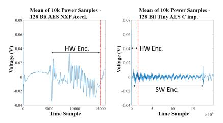
**Figure: 9.** Mean of 10k traces 20MHz @ core frequency. NXP crypthash accelerator running 128-bit AES (left), 128-bit tiny AES C implementation (right). The vertical red dashed line marks the end of the HW AES accelerator relatively to the SW one.
