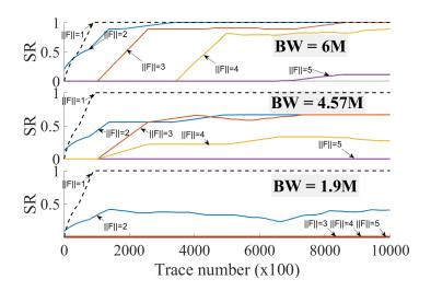
**Figure: 18. Risc-V SW Tiny-AES:** the success rate of a Gaussian template attack with varying ||F||. Black dashed line - no DVFS 20MHz, Blue - ||F|| = 2, Orange - ||F|| = 3, Yellow - ||F|| = 4, Purple - ||F|| = 5.
