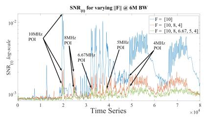
**Figure: 3.** Displaying with arrows when peak SNR values appear regarding to chosen  $f_n \in F$ , per case with different sized ||F||. The  $\Delta$  between the POI and the closest secondary peaks decreases, making it harder to choose a time sample for further analysis (i.e., template attacks).
