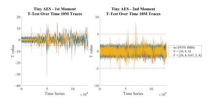
Figure: 15. Risc-V SW: example T-Test detection test based on TVLA methodology over time for 10M traces and for different ||F||, BW = 6MHz.
