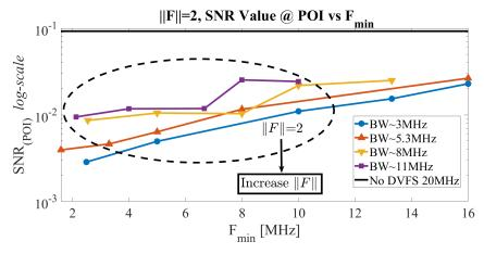
Figure: 14. SNR@POI values vs  $f_{min}$  for different BW.
