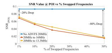
Figure: 25. Swapping from default 20MHz to a different core frequency for a percentage of the measured queries led to a reduction in the SNR POI value
